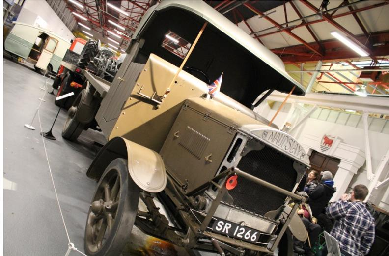
The Lorry was found in Scotland with a Fairground family and was just a chassis and engine in very poor condition. This model saw service with the RFC in Montrose, Scotland and was used as a general utility transport for the trainee pilots and observers.
